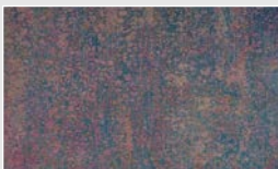
ISO 8501-1 锈蚀等级 B Sa1 Rust Grade B Sa1
