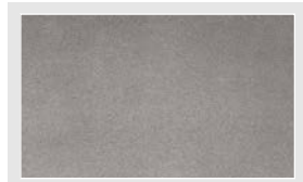
ISO 8501-1 锈蚀等级 B Sa3 Rust Grade B Sa3
