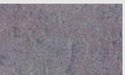
ISO 8501-1 锈蚀等级 B Sa2 Rust Grade B Sa2
